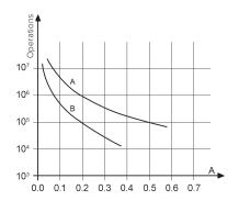
Contact loading: 110Vdc, L/R 40 ms Curve A: RCM.x6, RDM.x6 Curve B: RCM.x2, RDM.x2
